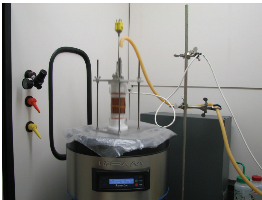
Figure 1. Photo showing setup of the acoustic mixer with column jacketed with electrical heat tracing. The vacuum line and temperature probe can be seen protruding from the top-end cap.
