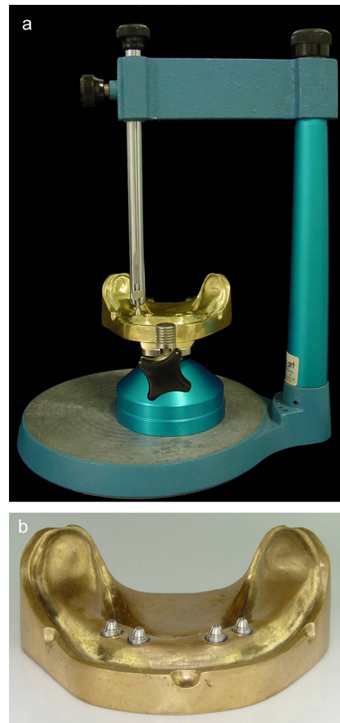
Fig. 1. Installation of the four parallel implant analogs with Duralay resin on master cast: (a) delineator confirming the parallelism between the implants analogs; (b) analogs fixed with Duralay resin.
