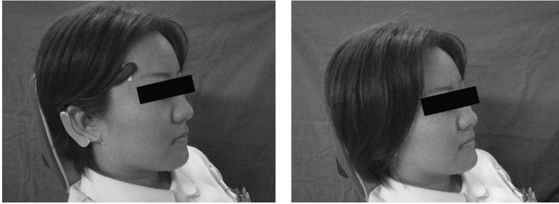
Fig. 1. The newly developed portable EMG recording and biofeedback system. Left panel: at completion of the apparatus set-up. Right panel: the apparatus is covered by the subject's hair.
