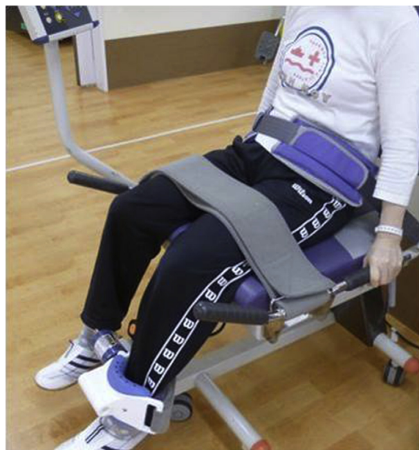
Fig. 1. Measuring the knee extensor and flexor strength. The knee extensor and flexor strength were assessed using IsoForce GT-330. With the patient in a sitting position with the hip and knee at an angle of 90°, the force sensor was placed over the anterior part of the lower leg 5 cm above the lateral malleolus. The seat position was adjusted for the length of the legs of each patient to allow him/her to push the pedal as hard as possible.
