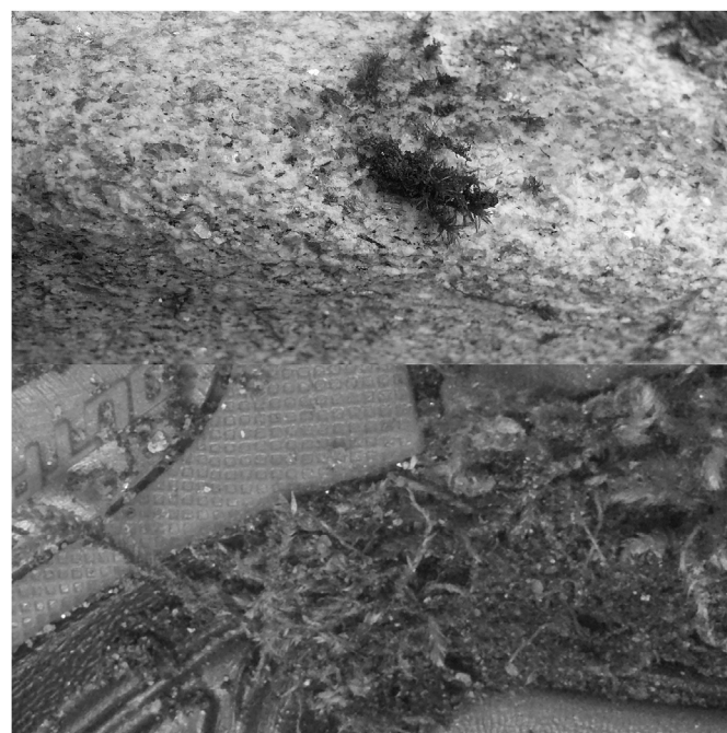
Fig. 2. Traces of removed mosses on the masonry parapet of the terrace (up) and under the shoes of the victim (down).
