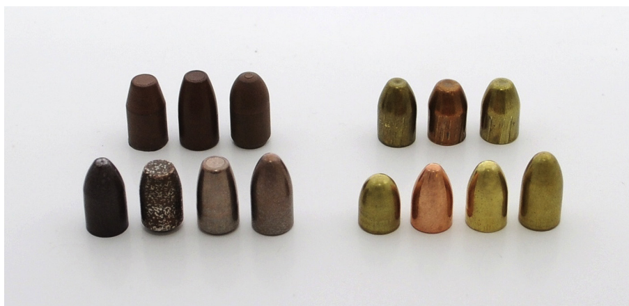
Fig. 2. Appearances of frangible projectiles (left) and classical full metal jacketed projectiles with a lead core (right). The back row on the right shows three fired projectiles, with deformation of the frontal part and grooves from the barrel rifling (all projectiles are for a 9 mm Luger pistol).
