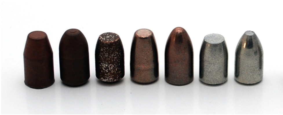
Fig. 1. Different types of 9 mm Luger pistol projectiles. The five projectiles on the left were made with copper powder, and the two projectiles on the right were made with iron powder.
