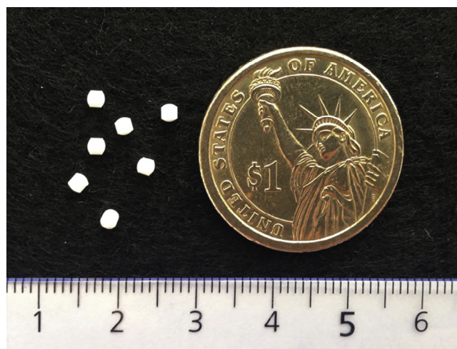
Figure 1. Dimensions of uncoated 2-mm diameter minitables (left) in relation to a $1 US coin (right).
