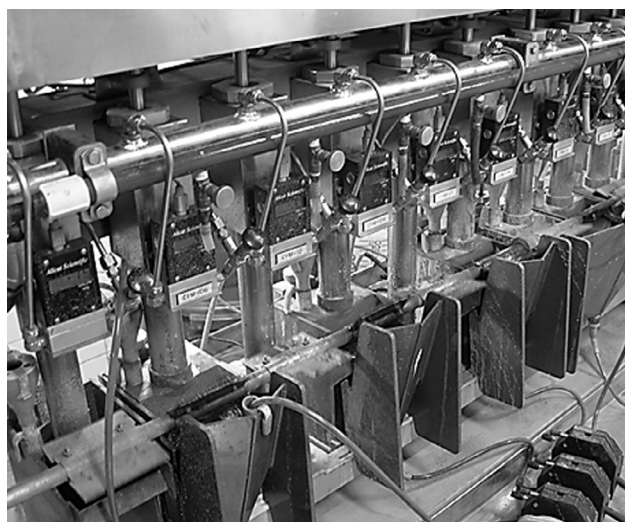
Fig. 1. Sequence of cells in the flotation mini pilot plant.
