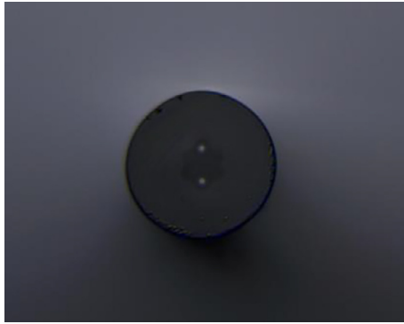
Fig. 2. Microscope image of the cross section of TCF.
