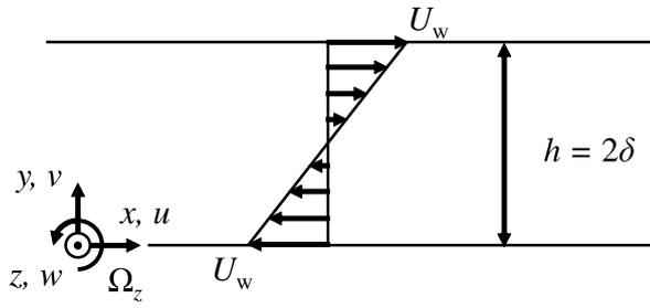
Fig. 1. Configuration of the rotating plane Couette flow.
