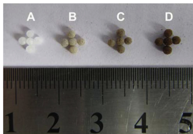
Fig. 1. The morphology of urea granule (A), fertilizer core (B), fertilizer coated with CAB (C), and LMF (D).
