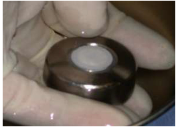
Fig. 1. Oxygen sensor array with integrated wireless telemetry system at implantation. The electrodes are imbedded into a ceramic disc that is hermetically sealed into the titanium housing. The electrodes are covered by a PDMS membrane. The implant is 3.4 cm in diameter and 1.5 cm thick.
