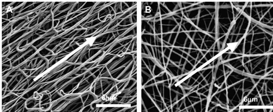
**Fig. 1.** Partially aligned (A) and random (B) electrospun PCL nanofibrous scaffolds. Arrow shows rotation direction of the mandrel.
