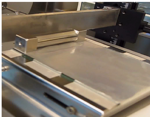
Fig. 2. The picture of the coating system, consisting of a doctor blade motorized by a linear motor system and home-made supporting stage.
