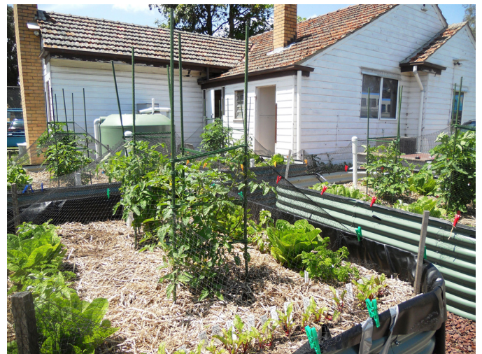
Fig. 1. Field trial raingardens; the Lined in the foreground and the Unlined to the right of the photo, with the two control gardens and the tile roof in the background. Each of the four gardens was constructed using a pre-fabricated modular raised garden bed made of corrugated steel. The four gardens were arranged in a non-random quadrant formation.
