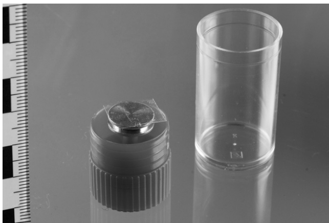
Fig. 1. Photograph of the modified SEM stub. It consists of a plastic container and holder, which contains an aluminum short pin stub holder to which the tape was attached. The holder is 2.5 cm high and ensures distance between investigator and trace.
