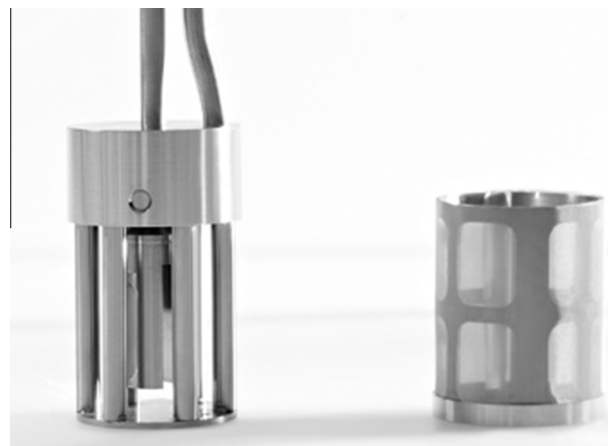
Fig. 2. Ultrasound sensor with crystallization adapter and exchangeable membrane (with kind permission of Senso Tech GmbH, see Nitschke et al. [16]).
