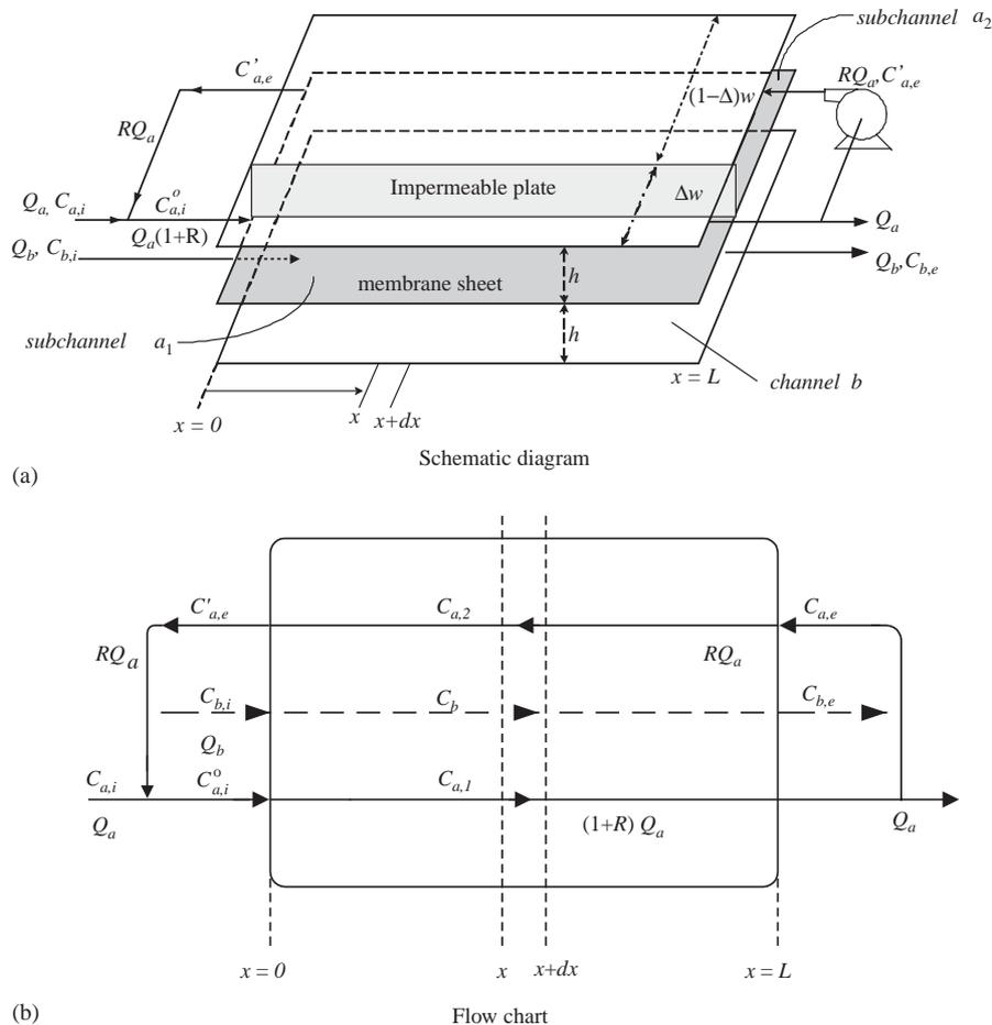
Fig. 1. (a,b) Parallel-plate membrane extractor with concurrent-flow operation and countercurrent-flow reflux.
