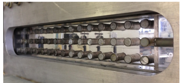
Fig. 3. Photograph of optical channel equipped with 12.7 mm diameter inline cylinders.
