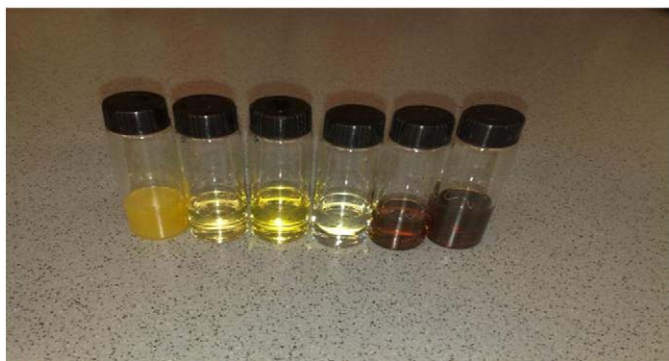
Fig. 1. Variation in color of condensate oils. Left to right: Waxy (BDR Co.); light yellow (Wapco-Ast-2); yellow (Khalada); colorless (Centurion-Azher); light brown (Petrobel-Fayroyz) and brown (Centurion-El-bassant-2).
