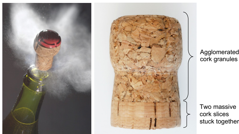
Fig. 1. Stop-action photograph of a cork popping out of a champagne bottle (Photograph by Jacques Honvault) (a), and side view of a traditional champagne cork stopper freshly-uncorked from a standard champagne bottle used in this set of experiments (b); it clearly appears that it is composed of two different parts: (i) an upper part composed of agglomerated cork granules, and (ii) a lower part made of two massive cork slices stuck together (Photograph by Gérard Liger-Belair).
