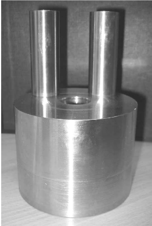
Fig. 1. Loading tool with punches. Die dimensions d_o=100 mm, d_i=25 mm, length=74 mm.
