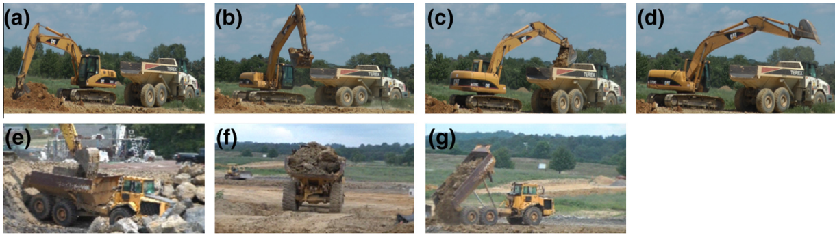
Fig. 1. Example frames from video sequences in excavator and truck action video dataset. Excavators: (a) digging; (b) hauling (swinging with bucket full); (c) dumping; and (d) swinging (bucket empty); Trucks: (e) filling; (f) moving; and (g) dumping.
