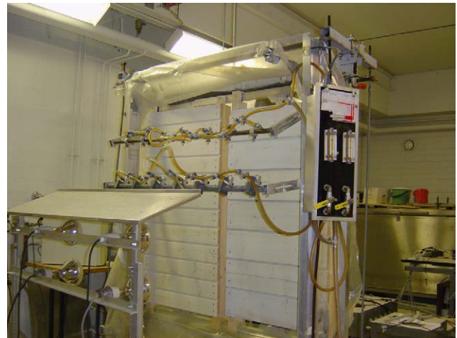
Fig. 2. Driving rain test apparatus and 2 test walls from the front.
