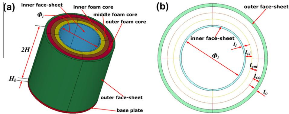
Fig. 1. Schematic of graded sandwich-walled hollow cylinder without cover: (a) overall view; (b) top view (base plate masked for better view).
