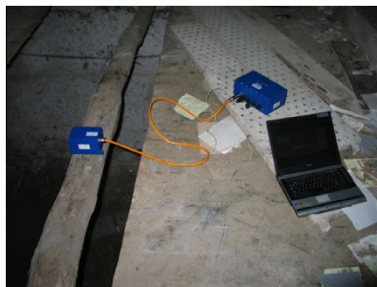
Fig. 1. Frequency measurement on a single timber beam.
