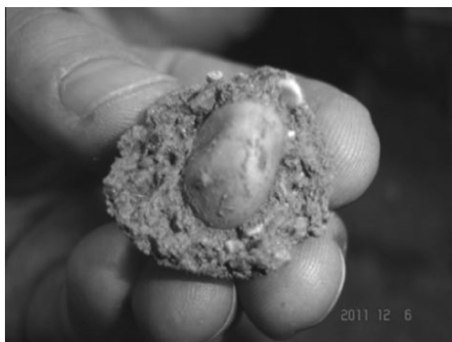
Fig. 1. Typical aspect of a fresh granular material after the addition of SAP.
