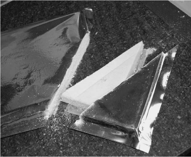
Fig. 1. Section of a VIP. The nano-porous fumed silica material is pressed in a PE fleece and sealed in a three-fold metallized polymer envelope under vacuum (below 1 mbar).
