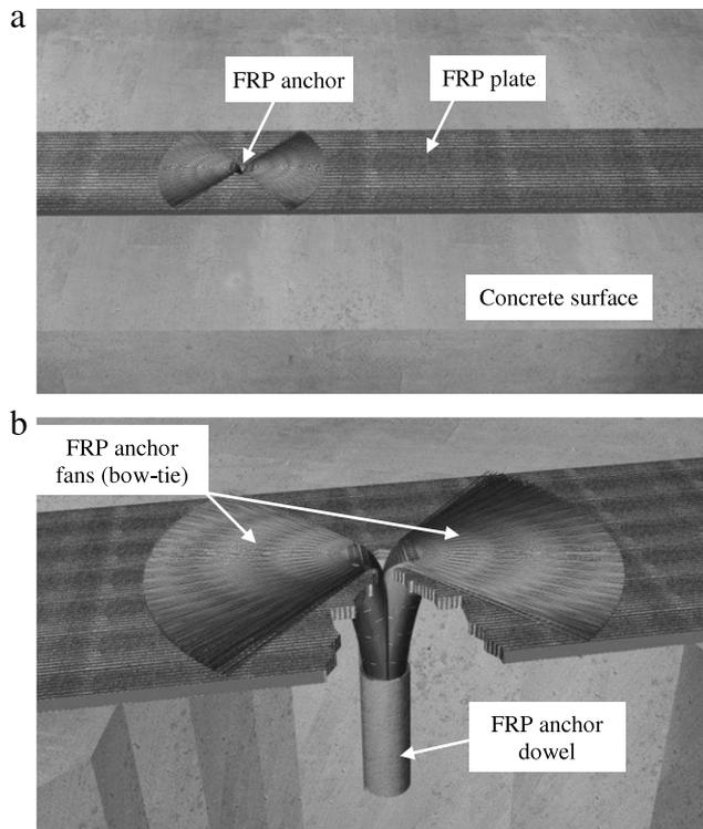
Fig. 1. FRP anchor and plate: (a) overall view; (b) cut-away view.
