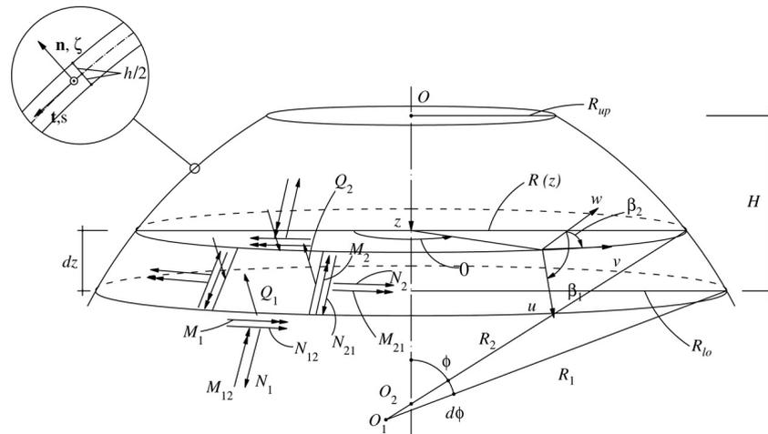
Fig. 1. Shell geometry and coordinate system of the reference middle surface.
