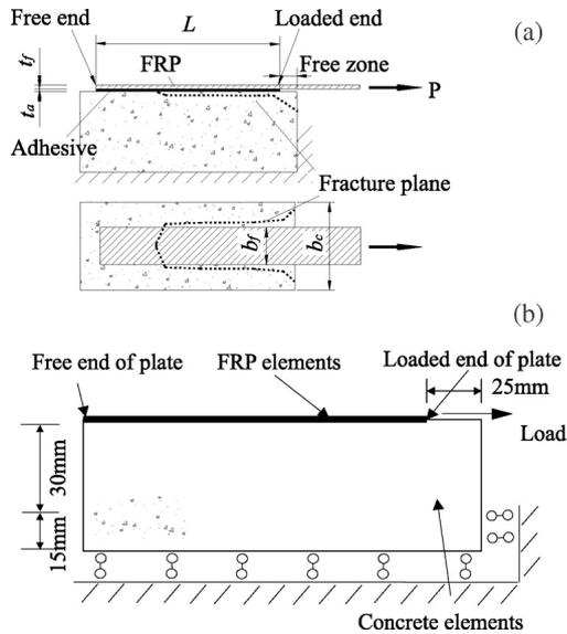
Fig. 1. Pull test: (a) Schematic; (b) FE model.
