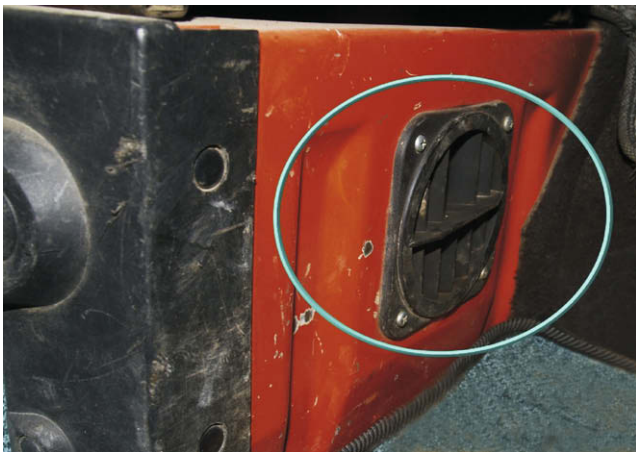
Fig. 2. Supplementary heater of the truck (case 1).
