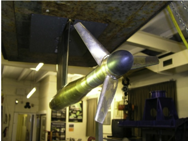
Fig. 2. Scaled tidal turbine model mounted on the dynamometer of Emerson Cavitation Tunnel [19].
