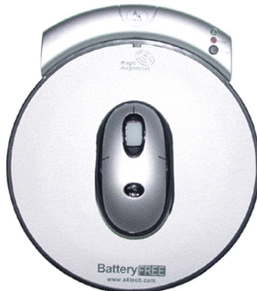
Fig. 1. The Battery-free wireless mouse (A4Tech, 2010) does not need batteries to keep it powered up (i.e. battery-free operation). It comprises a Radio Frequency Identification (RFID) mouse pad and its partner – a wireless mouse. The RFID mouse pad transfers necessary power to the wireless mouse through electromagnetic induction – RFID technology (RFID.org, 2010; Wikipedia, 2009a), and receives the wireless mouse operation signal via wireless connection to the computer. Simply placing the wireless mouse on the RFID mouse pad allows the wireless mouse to receive instant and constant power from the RFID mouse pad and work like a standard wireless mouse.
