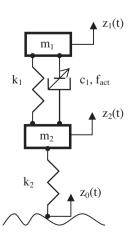
Fig. 1. Quarter car model with semi-active suspension.
