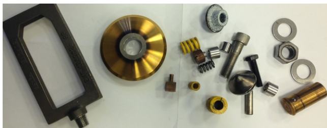
Fig. 2. Typical solid waste material produced from nuclear plant decommissioning process (National Nuclear Laboratory and Sellafield Ltd, UK).
