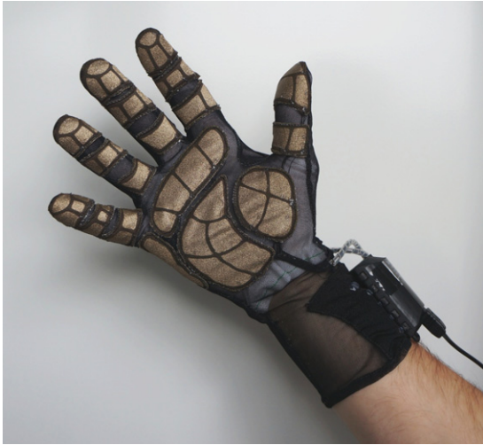
Fig. 1. Wearable dataglove with 54 tactile cells and embedded data acquisition electronics. It utilizes novel fabric based tactile sensors.
