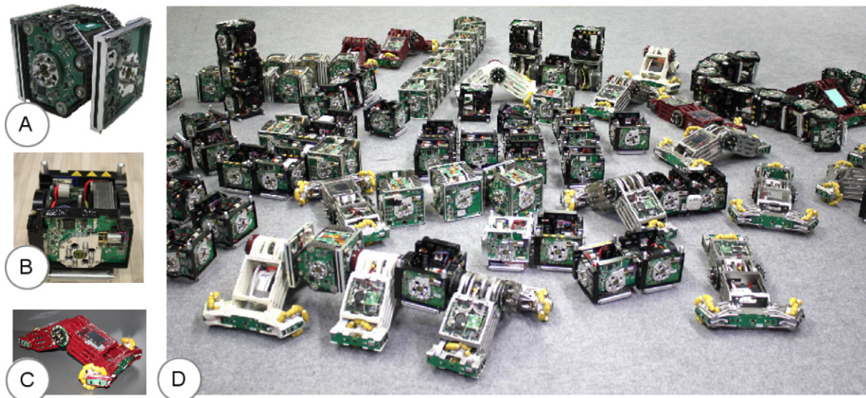
Fig. 1. Three different robot modules were constructed: (A) Scout [11], (B) Backbone [12], and (C) Active Wheel [13]. All three are equipped with different sensors and actuators. (D) Shows a swarm of single robots and already assembled organisms collected in our in-door arena of 35 m 2 . It is characterized by different zones containing ramps, gaps, various flooring styles, and power sockets that are installed at various heights (these zone are clearly visible in Figs. A17, A18 of the supplementary material, Appendix A).
