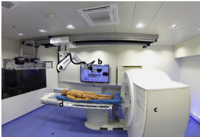
Fig. 1. A Virtobot during a demonstration: a. robotic arm, b. Nikon D700 camera, c. CT, and d. CT table. The robotic arm rotates around the dummy to capture images from each of the 25 standard positions with the Nikon D700 camera. Data are fed directly into the ATOS Professional software.
