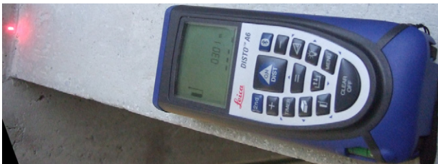
Fig. 2. Leica Disto laser range finder with 1–2 mm precision over 60 m.
