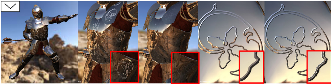
Fig. 1. The Knight Champion rendered from different viewpoints and distances using our approach (left images, 59–78 fps) and relief mapping (right images, 57–81 fps) to simulate the armor engravings. Observe how our antialiasing strategy correctly reproduces the grooves visibility while relief mapping produces noticeable artifacts (insets).
