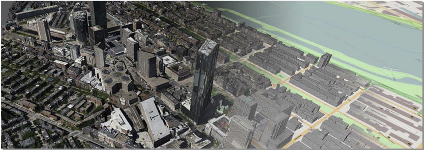
Fig. 1. Urban modeling. A complex urban area (left) is automatically obtained using volumetric reconstruction with surface graph cuts (middle) computed from aerial imagery and GIS-style parcel/building data (right). Our methodology uses photo-consistency to robustly recreate 2.5D building structures and surface graph cuts to assemble seamless and coherent textures despite occlusion, geometry, and calibration errors.
