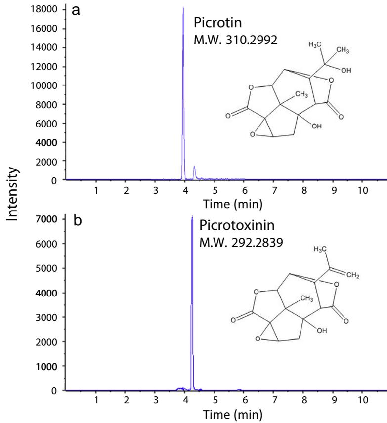
**Fig. 1.** Mass chromatograms of **a** picrotin at  $m/z$  309.098 and **b** picrotoxinin at  $m/z$  337.094 in the MS mode; 0.26 ng on-column of each compound was subjected to LC-Q-TOFMS.
