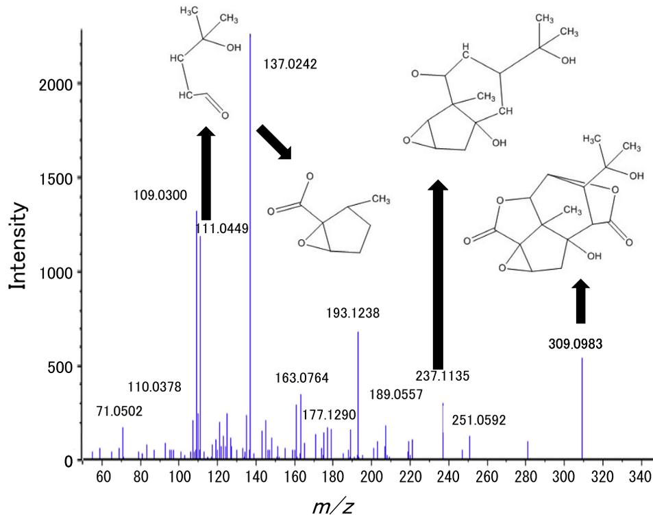
**Fig. 2.** The MS/MS spectrum of picrotin (2.6 ng on-column). Possible structures of fragment ions are shown in the inset.
