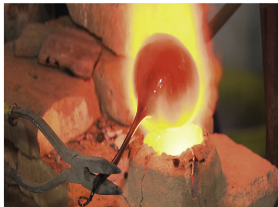
Fig. 2. Drawing of a glass tube according to the lada method (Gudo, Indonesia). Photo J.W. Lankton.
