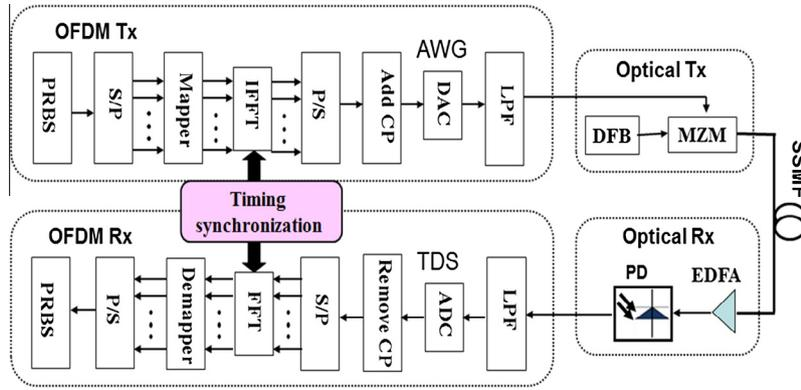
Fig. 1. Principle of DD-OOFDM transmission system. Tx: transmitter; LPF: lowpass filter; Rx: receiver.
