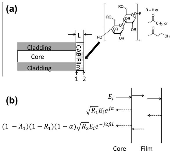
Fig. 1. (a) Structure of the sensing head and the molecular structure of CAB and (b) the field amplitude at the reflection interfaces,  $R_1$ ,  $R_2$  respectively represent the reflection coefficients from interface 1 and 2.
