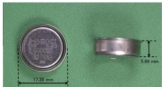
**Fig. 1.** Appearance of the button-type thermo data logger.
