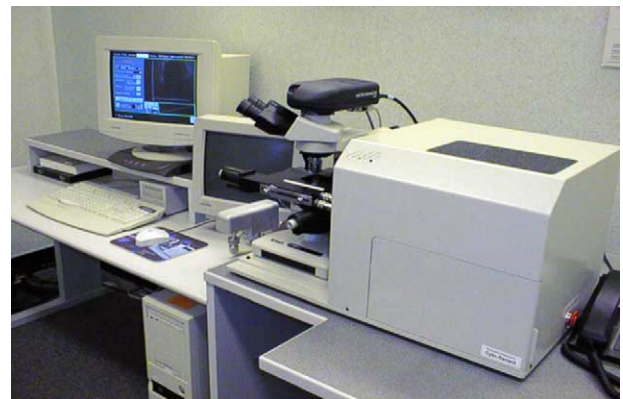
Fig. 2 Cytosavant® is a computer-assisted image analysis system for the quantitative measurement of cytopathology and histopathology. The system consists of an autofocusing microscope, two computers, and an automatic slide loader.
