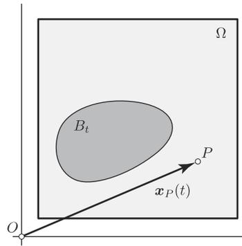
Fig. 1. Current configuration  $B_t$  of a body  $\mathcal{B}$  immersed in a fluid occupying the domain  $\Omega$ .
