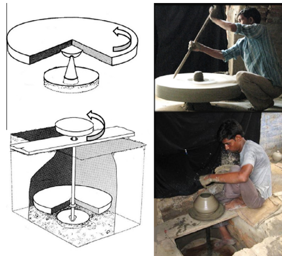
Fig. 1. The two common wheels used in northern India. Top panel: the high inertia stick-wheel used by the Prajapati potters. Bottom panel: the low-inertia kick-wheel used by the Multani potters. Drawings are adapted from Orton et al. (1993). The two wheels evoke distinct body positions: for the stick-wheel potters typically squat (sometimes they use a low stool), while for the kick-wheel potters sit.
